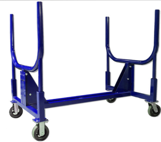
Rolling Cradle (ME-68U) - The rolling pipe cradle is specifically designed to transport large bundles of conduit, pvc and copper pipe, small bore steel pipe and threaded rod in one large cradle. Dimensions- 56"Lx34"Wx34"H. Capacity: 1,000 lbs.
